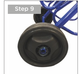
Step 9: Position wheels (M) onto axle and gently hammer spring clips (N), one each side of reel, onto the axle, clips facing outwards, until wheels are held securely with no lateral movement.
